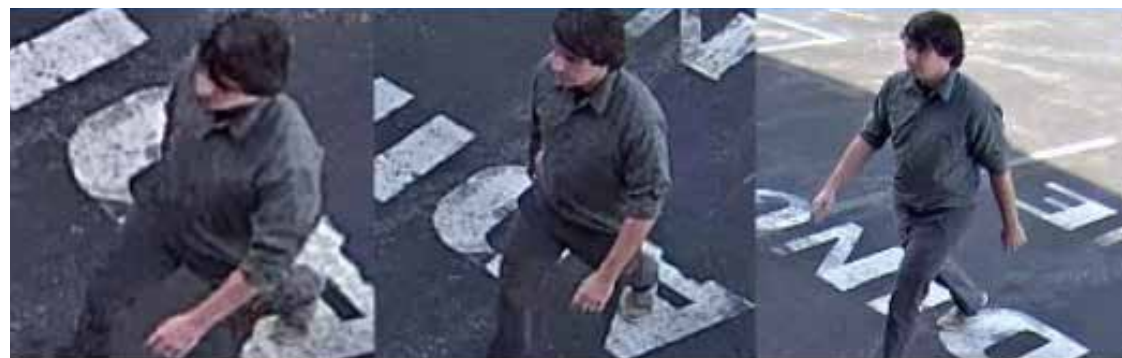
Research CCTV demonstration by IPVM shows that above certain heights facial details start to be lost and subjects can easily conceal their face when tilting their head
