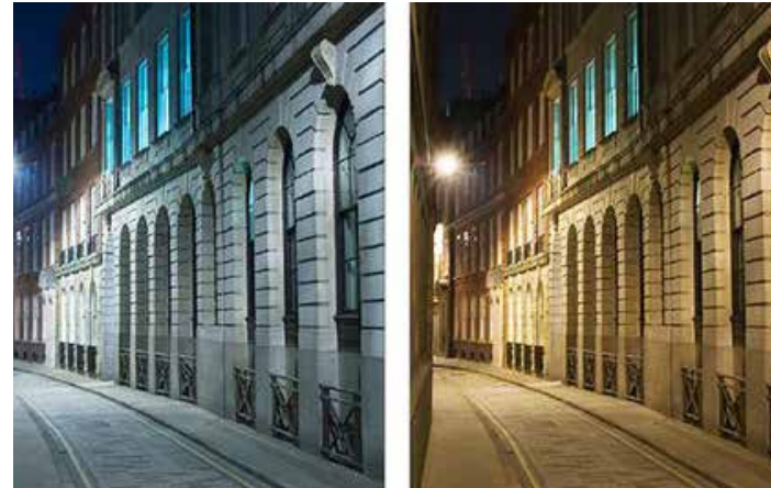
Test showing the effect of colour temperature on a streetscape environment ©Speirs and Major
