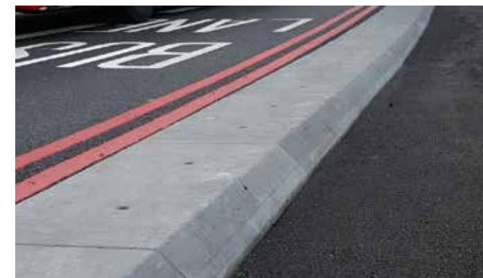
The cycle segregation kerb by Charcon has a half batter along the carriageway, capable of withstanding vehicular impact and a splay edge on the carriageway side, which significantly reduces the chance of cyclists catching a pedal.
